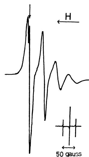
Fig. 5. ESR spectrum of Cu-PTTU in \text{CH}_2\text{Cl}_2 -EtOH solution at 15^\circ\text{C} . The arrow indicates the resonance field for DPPH ( g=2.00354 ).
